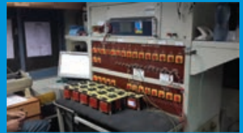
QUALITY ASSURANCE CONTROL / VOLTAGE TRANSFORMER TEST BENCH
